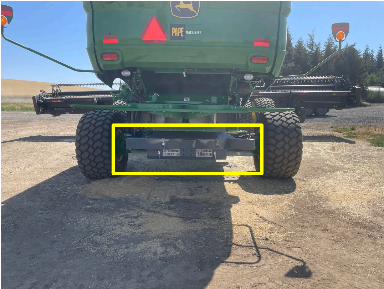
Figure 23. A Seed Terminator unit mounted on a combine for harvest weed seed control. July 2023. Whitman County, WA.
