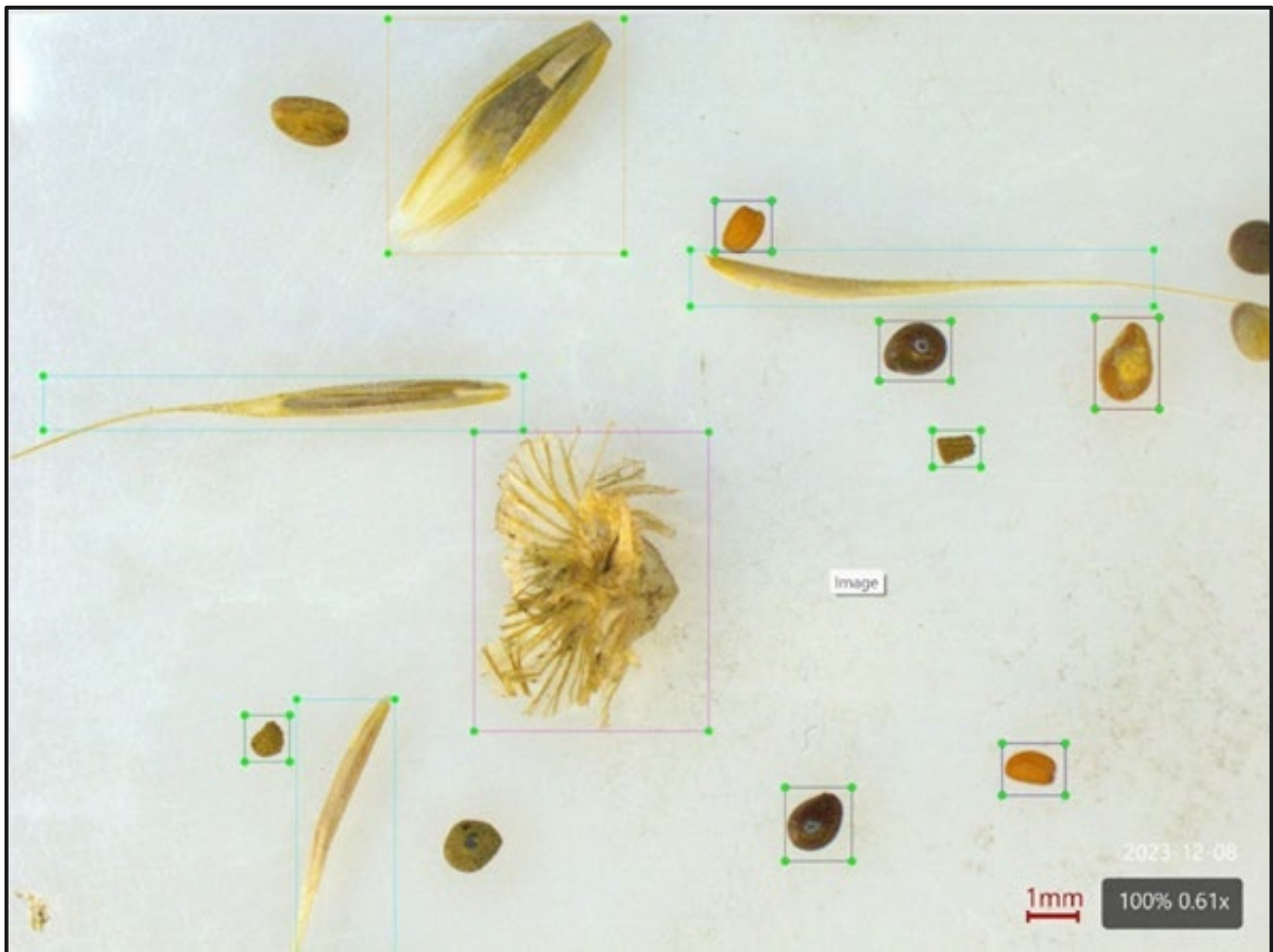
Figure 17. labelling generated bounding boxes drawn around weed seeds belonging to different classes used in the training process
