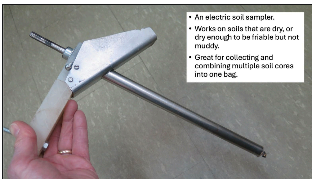
Figure 2. Weed seed bank sampling apparatus that will be used at each site.
